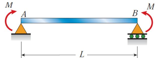
$$U = \frac{1}{2} \int_V \frac{M_z(x)^2}{EI_{z,y_0}^2} (y - y_0)^2 \, dx \, dy \, dz \quad \rightarrow \quad I_{z,y_0} = \int_A (y - y_0)^2 \, dy \, dz$$
