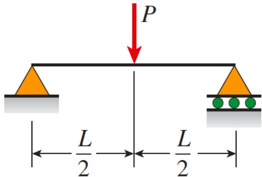
$$v = -\frac{Px}{48EI} (3L^2 - 4x^2) \quad v' = -\frac{P}{16EI} (L^2 - 4x^2) \quad \left(0 \leq x \leq \frac{L}{2}\right)$$
